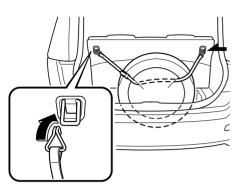
11. Pull the belt end to secure the flat tire.
